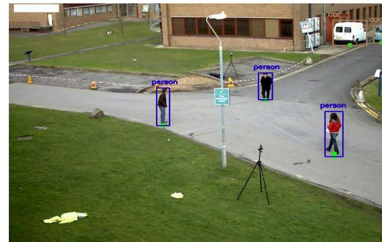
Figure 4. Bounding boxes drawn on an original frame from the result of the YOLOv5 neural net
