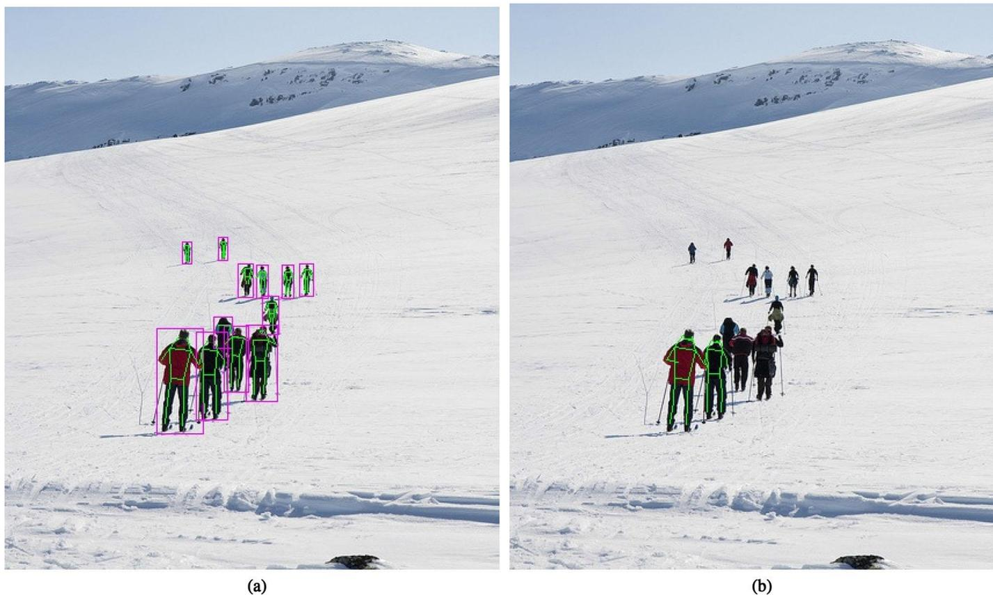
Figure 8. A comparison from the CrowdPose dataset showcasing superior performance of our method on far away pedestrians: a shows output from our method (YOLOv5 bounding box and OpenPifPaf pose estimation); b shows output from DEKR [14]
