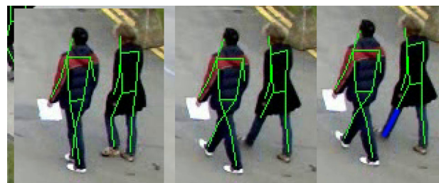
Fig. 10 Left shows the previous frame where the complete leg is detected. Middle shows the current frame where the lower leg is not detected by OpenPifPaf. Right shows the lower leg estimation in the current frame using our pedestrian localization technique
