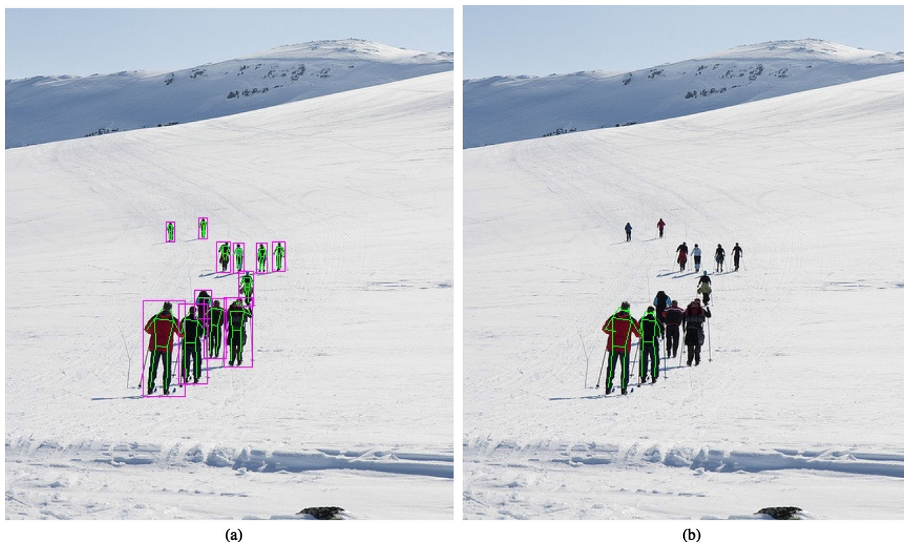
Fig. 8 A comparison from the CrowdPose dataset showcasing superior performance of our method on far away pedestrians: a shows output from our method (YOLOv5 bounding box and OpenPifPaf pose estimation); b shows output from DEKR [14]
