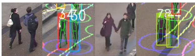
Fig. 17 People seen talking with each other and holding hands are detected as together by the smart violations detector
