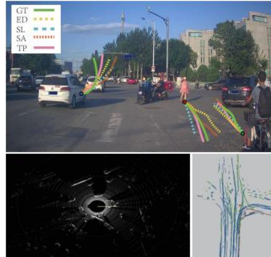
The green solid lines denote ground truth trajectories (GT), pink solid lines are for paper method (TP) and dashed lines are the predicted trajectories for other methods (ED, SL, SA)
